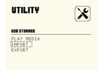
3). Use direction button to select <u>IMPORT</u>, then press **[ENTER]** button to enter into import interface;
