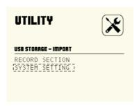
4). Use direction buttons to select <u>SYSTEM SETTING</u>, then press **[**ENTER**]** to import USB user drum kit information.
