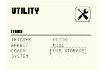
C. In UTILITY interface, use direction buttons to select <u>USB STORAGE</u>, then press [ENTER] button to enter into USB setting interface;
